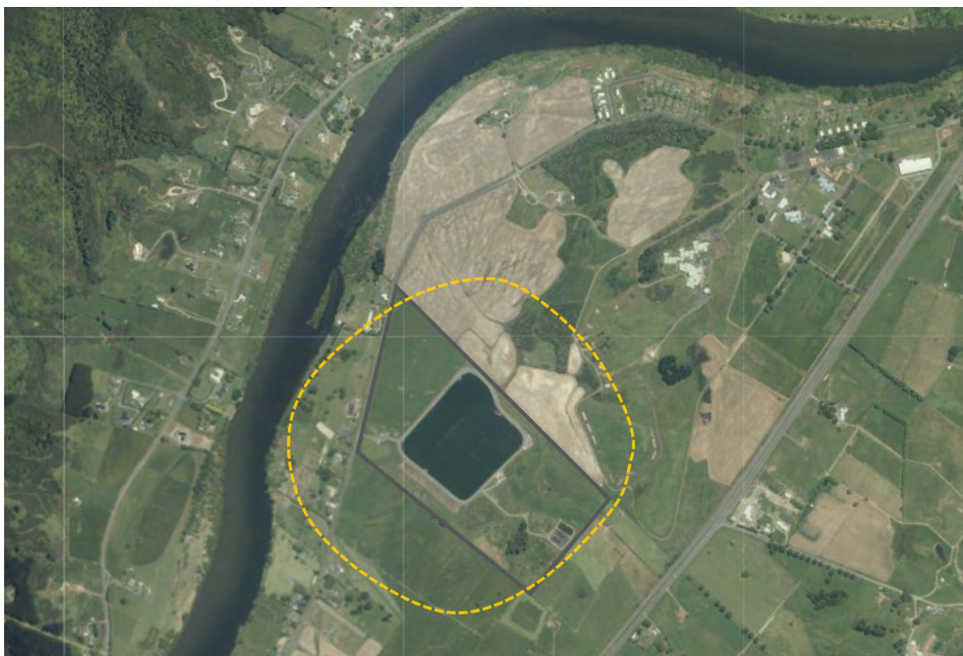
Figure 11: Approximate 300m buffer from oxidation pond (yellow dash). This buffer zone extends outside the WDC-owned property shown in grey.
